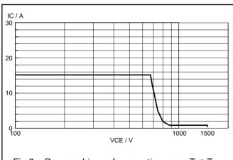
Fig.9. Reverse bias safe operating area.  $T_j \le T_{jmax}$
