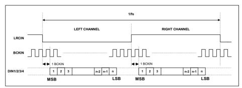
Figure 13 I<sup>2</sup>S Mode Timing Diagram
