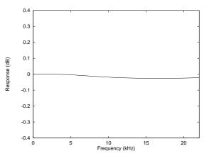
Figure 24 De-Emphasis Frequency Response (44.1kHz)
