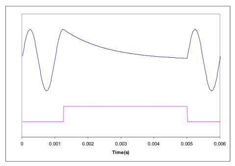
Figure 17 Application and Release of Soft Mute
