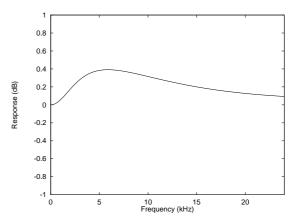
Figure 26 De-Emphasis Frequency Response (48kHz)
