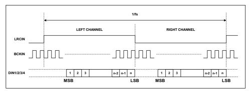
Figure 12 Right Justified Mode Timing Diagram
