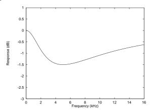
Figure 22 De-Emphasis Frequency Response (32kHz)
