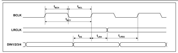
Figure 5 Digital Audio Data Timing – Slave Mode
