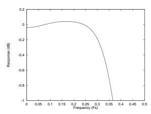
Figure 20 DAC Digital Filter Frequency Response – Figure 21 DAC Digital filter Ripple – 192kHz 192kHz
