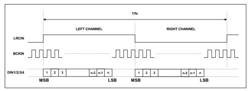
Figure 11 Left Justified Mode Timing Diagram
