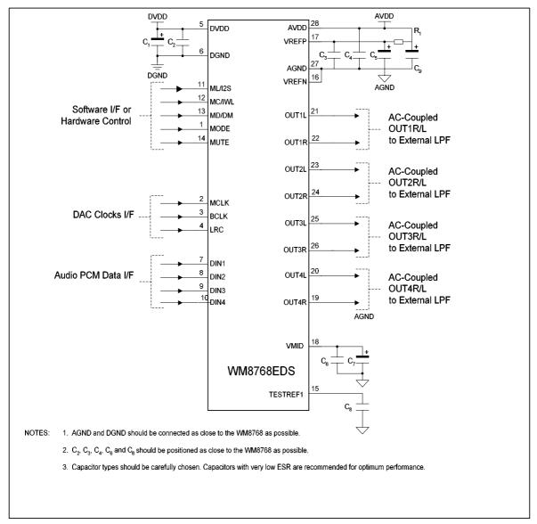
Figure 28 Recommended External Component Diagram
