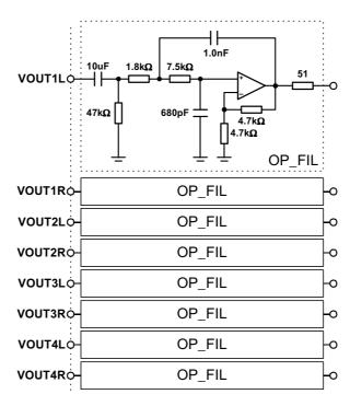
Figure 29 Recommended Post DAC Filter Circuit
