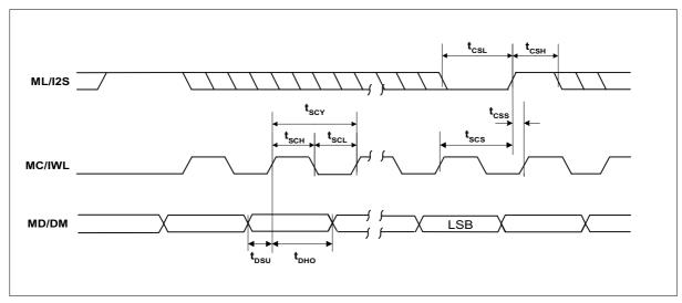
Figure 6 SPI Compatible Control Interface Input Timing
