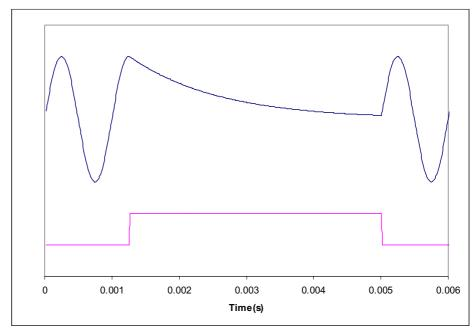
Figure 7 Application and Release of Soft Mute
