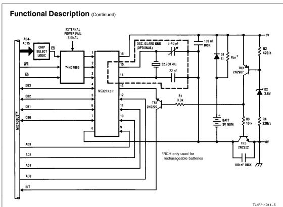
FIGURE 3. Typical System Connection Diagram
